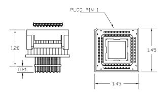
Press rim to open socket, press device to close
